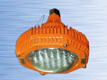
2 models available **CERTIFICATION:** Titan Pendant Titan 24V Pendant 5820 Lumens 80° beam ATEX MODE High CE Œ 100-277V AC 24V IP66 0000 Ĵ 220 x 220mm 10.4kg EC Ray SA-TITAN-PENDANT SA-TITAN-PENDANT24 CODE
