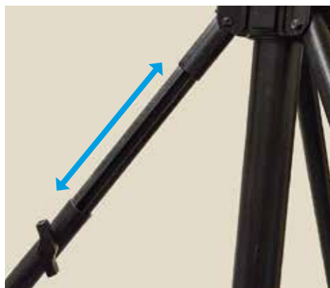
Extendable tripod leg for uneven slopes
